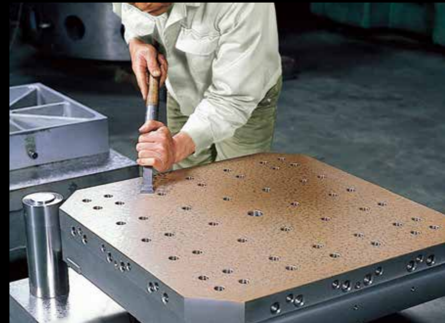
Hand scraping on the master jig plate
