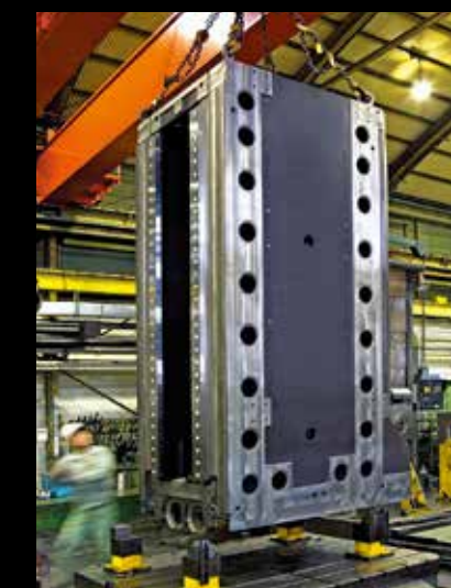
Column in the double housing structure
