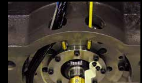
Cooling system of the ball screw bracket
