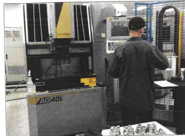
Phil Mendes, moldmaker, is working to set up one of the company's EDM cells so that it will run over the next couple of days. This cell comprises two Sodick AG40L sinkers with a carousel and System 3R Workmaster robot that feeds the two machines. Using automation has helped to significantly advance X-Cell's operations while also reducing costs and optimizing lead times.
