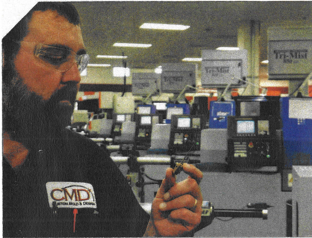
Swiss turning can quickly and accurately make long, thin parts like this core pin, and make most parts in a single operation without custom fixturing.
