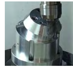
Circularity (Measured value) 2.82μm
