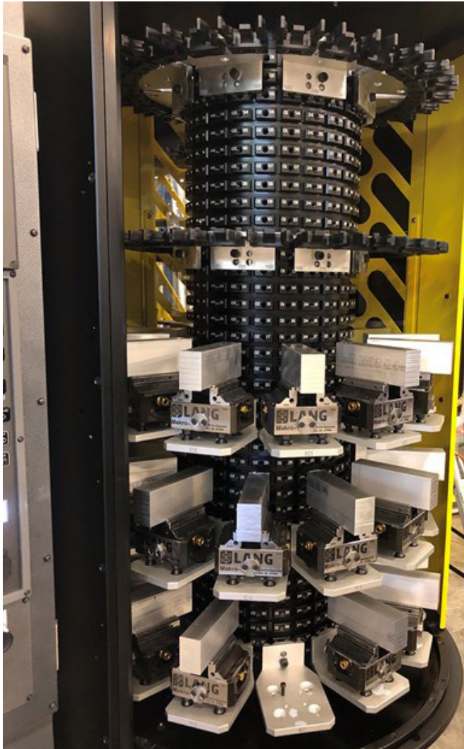
NRL is now producing a number of ventilator components for two customers. The more complex parts go in the multi-pallet FANUC Robodrill with Plus-K automation, shown here, or in one of its two Yasda PX-30is.
