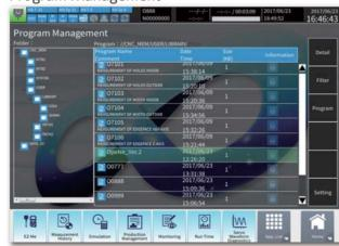
On this screen, machining time for any registered program can be easily calculated by simulation even while the machine is operating.
