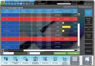
On this screen, not only basic tool information but also associated tool information such as machining load and measurement history are collectively managed.
