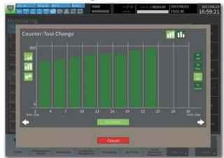
On this screen, various data such as number of operations and running status of peripherals are automatically acquired and saved. Use of acquired data allows for planned and efficient maintenance and predictive maintenance on equipment. A check if current machine status is appropriate or not is carried out automatically by acquiring servo wave data and comparing it with past data.
