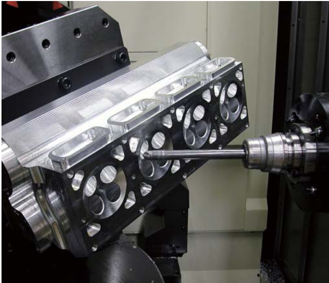
5-axis simultaneous machining for inlet/outlet holes
